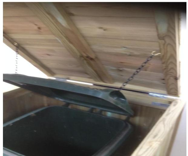
Hook one side of the chain to one of the hooks underneath the lid, slide the other end through both handles on your wheelie bin and attach to the other hook. The bin lid will be automatically open when the store lid is opened for easy filling.
